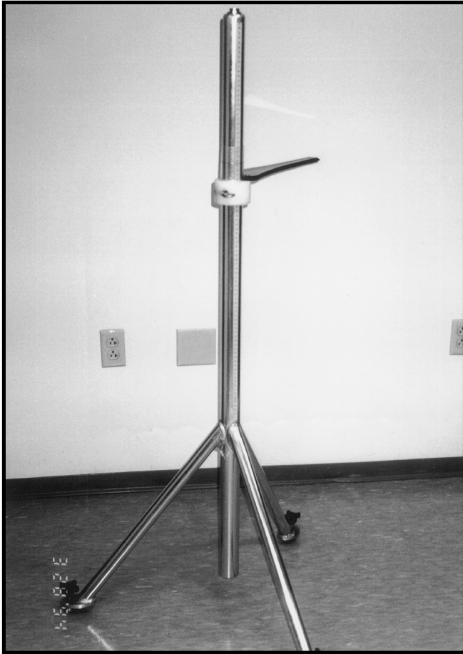
Figure 1. A pedestal-mounted post with an adjustable horizontal arm was used to measure heights of palpated landmarks (in millimeters).
